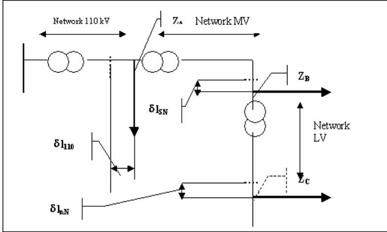
Figure 1 Diagram of the model distribution network
