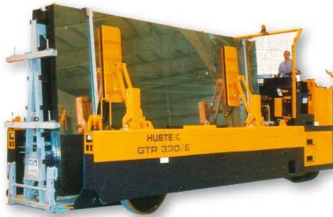
Figure 3. Truck made by Hubtex Company designed for shipment of glass racks [5.]
