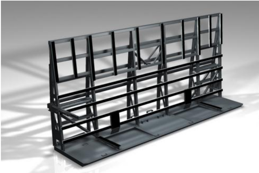
Figure 2. The rack for storage and transport of Jumbo-size glass sheets [4.]
