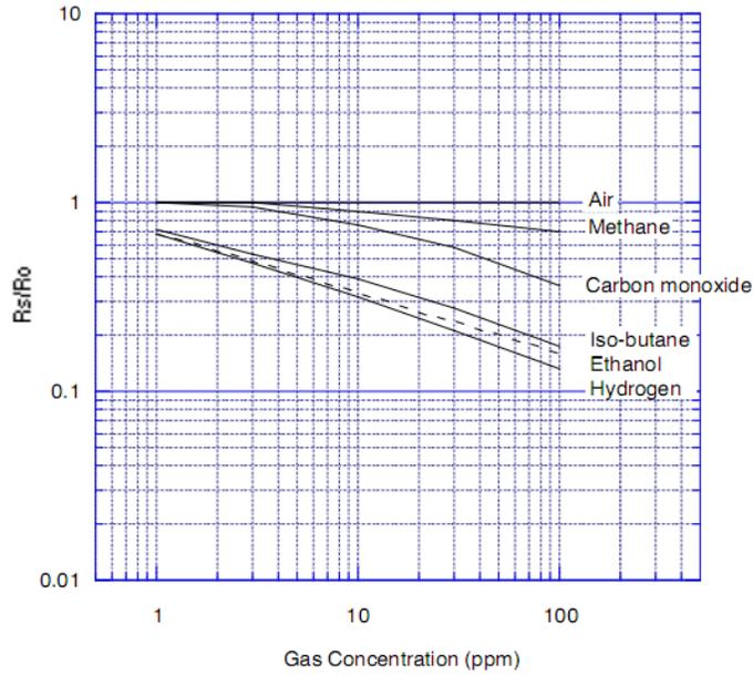
Figure 5. Characteristic of the TGS 2600 sensor [4.]
