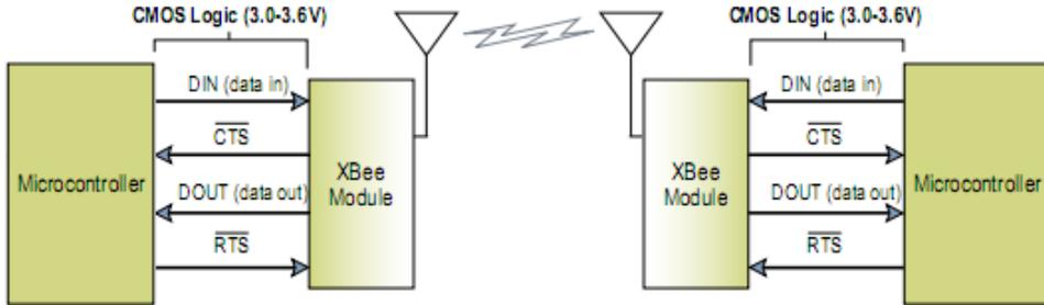
Figure 4. Microcontroller-xBee connection
